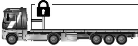
***When UNLADEN ensure the blade is restrained by a blade lock mechanism***
