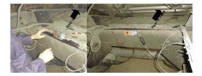
8. Mount the Sensor Cover over the Sensor Unit using four M5 x 40 HEX bolts. Use Silicone sealant or other waterproof sealant to make a waterproof seal between the Sensor Cover and the trailer cross member.
