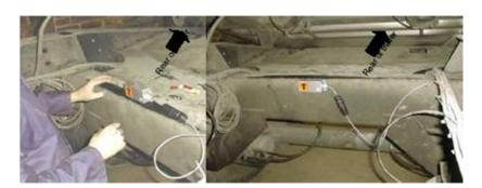
14. Mount the Sensor Cover over the Sensor Unit using four M5 x 40 HEX bolts. Use Silicone sealant or other waterproof sealant to make a waterproof seal between the Sensor Cover and the trailer cross member.
