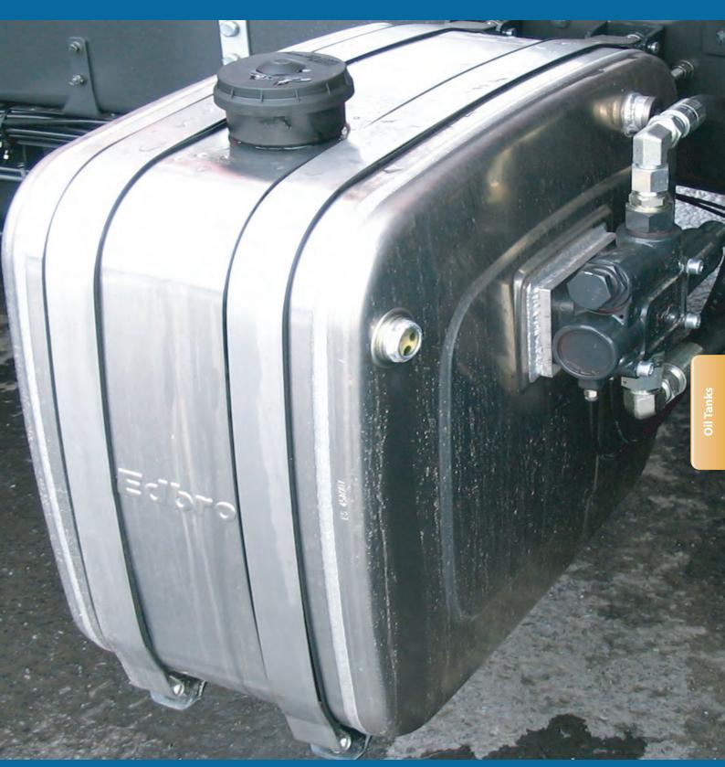
Edbro Oil Tanks are available in both aluminium and steel with a range of sizes and designs to suit all applications.
