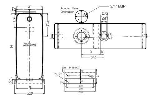
Top mounted valve plate for easy maintenance Compatible with Edbro valve CT200 Integral oil level sight glass Tanks finished in RAL7021 grey superior primer
