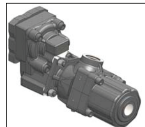
4 - Push the pump against the PTO and tighten the nuts fully home. The tightening torque shown in TABLE 3
