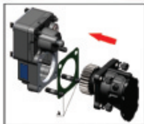
2 - After mounting PTO on the gearbox, screw the studs (pos.A) onto the PTO. Place the intermediate gasket and then fit the PTO assembly (fig 1) onto the PTO. Fix the pump applying the tightening torque indicated in TABLE 3.
