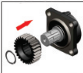
1 - Mount loose gear and circlip on the pump's shaft
