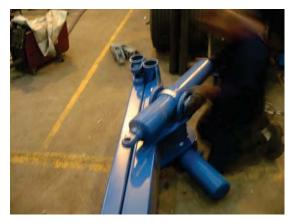
7. Align cylinder eye with top bracket, replace clevis pin and bolt, and tighten clevis pin bolts. Repeat for second cylinder
