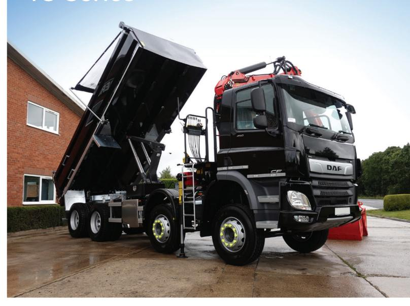
The Edbro TS range of twin underbody cylinders for unquestionable reliability in tipper & tipper/grab operations
